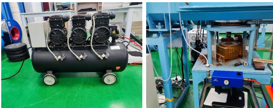
Fig. 2: Compressor and fog generator.
