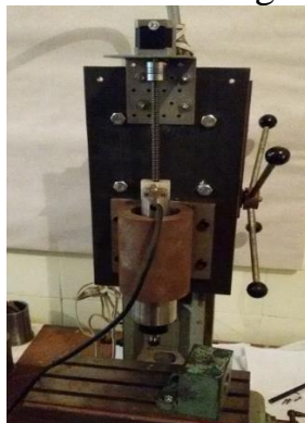
Fig. 4. Stand for experimental studies of self-acting M-S
